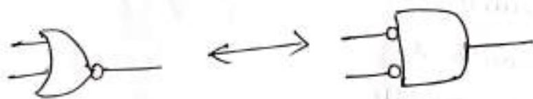
Figure :- Bubble pushing with DeMorgan's Law.
